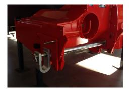
• The hitch's **semi-automatic** design facilitates coupling operations.
