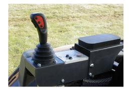
• HE (Hydraulic/Electric) type proportional joystick control. Combined pivot, main and outer booms, and cutting head movements are also possible.
