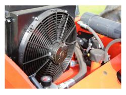
• Oversized oil cooler: **12 kW as standard,** offers constant power and protection of hydraulic components.
