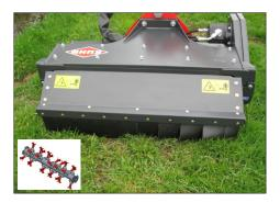
The head is **belt driven** and receives a **reversible rotor** (the rotor can thus be turned around to optimise lug wear). This rotor receives **60 "broad" Y-flails mounted on 14 mm shackles**. The assembly is driven by a sensor roller, measuring 140 mm in diameter, and with removable ends.
