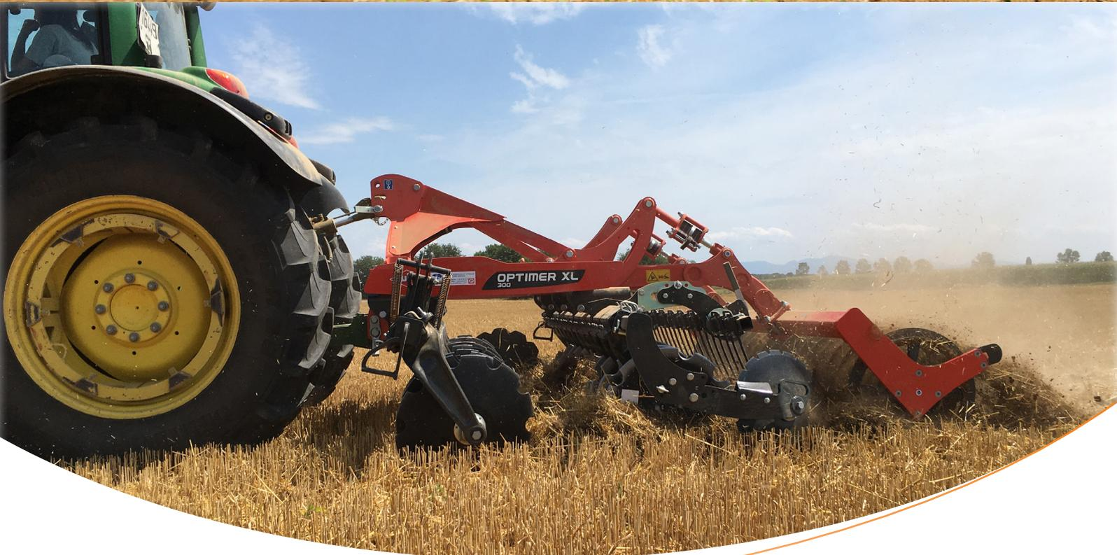
OPTIMER XL: intensive mixing at high speeds with **620 mm diameter discs**.
